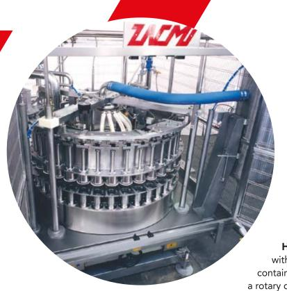
**Customized layout:** Vacuum Filler can be mechanically or electronically synchronized with all ZACMI Seamers.
